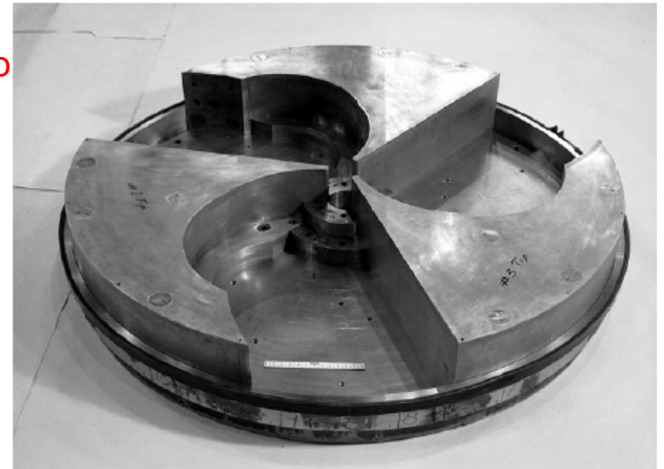
Spiral pole pieces of the Oak Ridge Isochronous Cyclotron (75 MeV)
